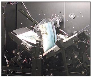
Page-handling technology developed for the Kirtas APT BookScan 1200. The V-shaped SmartCradle uses independently moving plates to precisely maintain the top pages of the book in the focal plane of the camera, while the Sure-Turn robotic arm uses a vacuum pickup head, edgedetection sensors, and puffs of air to reliably turn pages whose texture ranges from onion skin paper to photographic stock.
